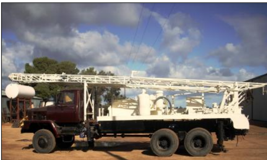
Mayhew 1000 series drill rig remounted to UD 6x6 truck base. Hydraulic levelling jacks and other equipment still to be fitted.
