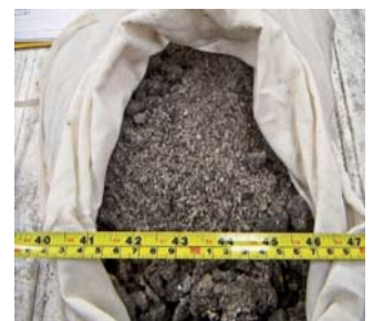
Uranium mineralised course grained sands drill hole MRM021, eastern mineralised zone
